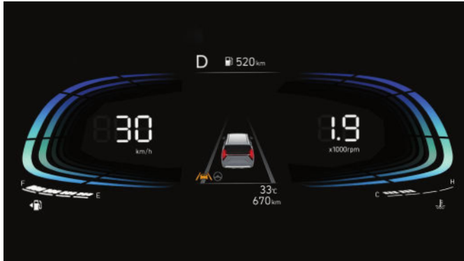
4.2" TFT Color + Full Segment LCD Cluster
