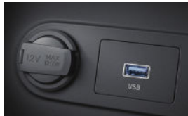
12 V Power Outlet + USB Multimedia Port
