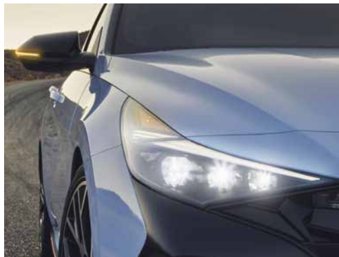
LED projection-type headlights LED daytime running lights LED mirror-mounted turn signals
