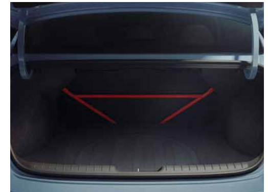
Rear strut bar offers an enhanced body rigidity increase of 29%, compared to the standard ELANTRA model
